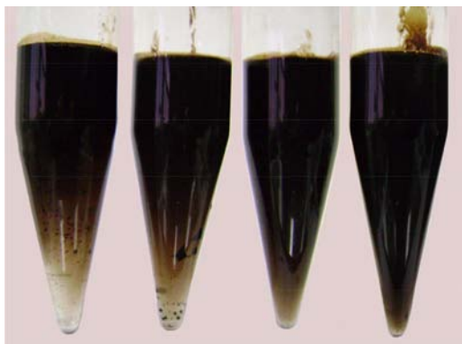
Fig. 7—HCPF produced emulsions after centrifuging during one group of bottle tests. (The water cuts are 80, 65, 55 and 40%, in order from left to right, and the polymer-containing concentration is 920 mg/L.)
