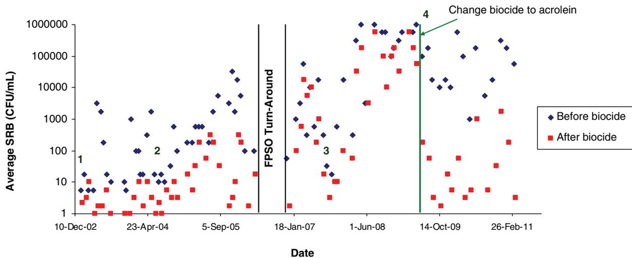
Fig. 6—Average SRB levels before and after acrolein biocide treatment on FPSO producer.
