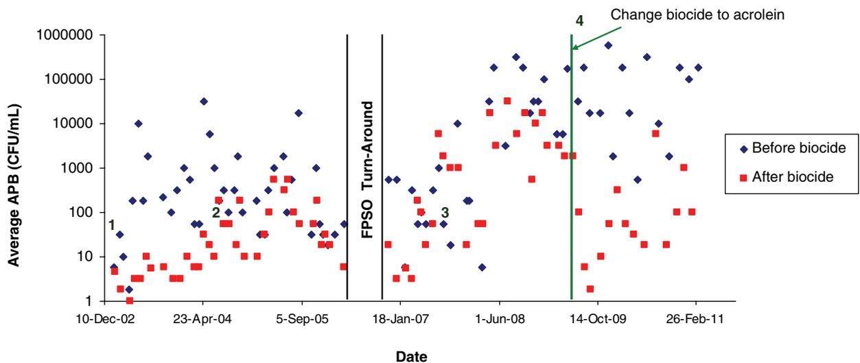
Fig. 7—Average APB levels before and after acrolein biocide treatment on FPSO producer.
