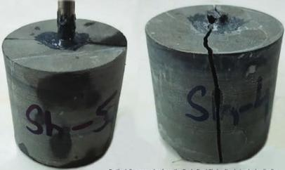
On the left, a core plug from the Eagle Ford shale after being hydraulically fractured with slickwater. On the right, another sample from the same formation that has been split in half using a new thermochemical formula that may displace large numbers of pressure-pumping units. Source: URTIC 2429.
